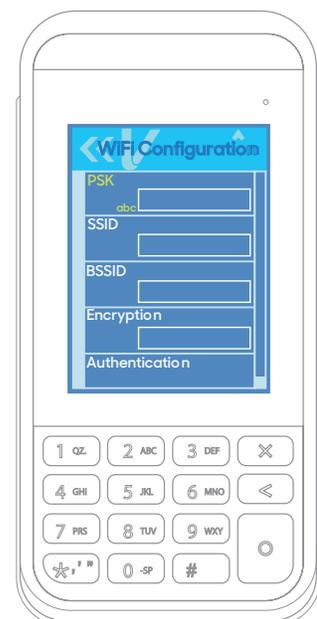
7. Tap **WiFi Configuration**. In the **PSK** field, type the network's password. To switch between lowercase letters, capital letters, and numbers press the **#** button.
